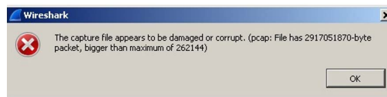
Figure 54-8: Example of a corrupted PCAP file loaded in Wireshark
