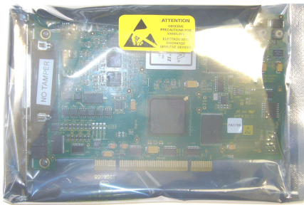
GROUND STATION BOARD
